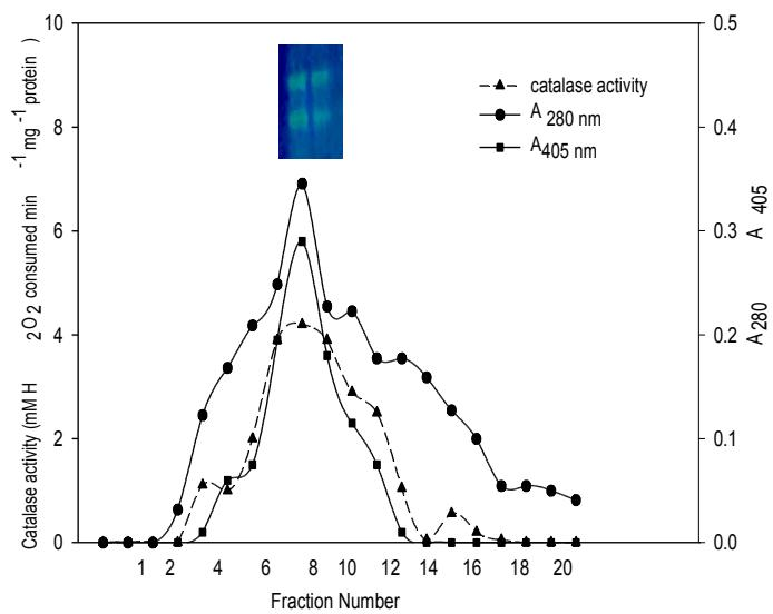
**Supplementary Fig.3a.** Gel-filtration chromatography of ethanol fraction obtained after ethanol: chloroform treatment during purification of catalase. The enzyme was eluted with 100 mM KPB (pH 7.0) at 30 ml h<sup>-1</sup> flow rate and 2 ml fraction volume. (Inset: Native-PAGE of catalase isoforms from pooled fractions 7-12 with maximum enzyme activity).
