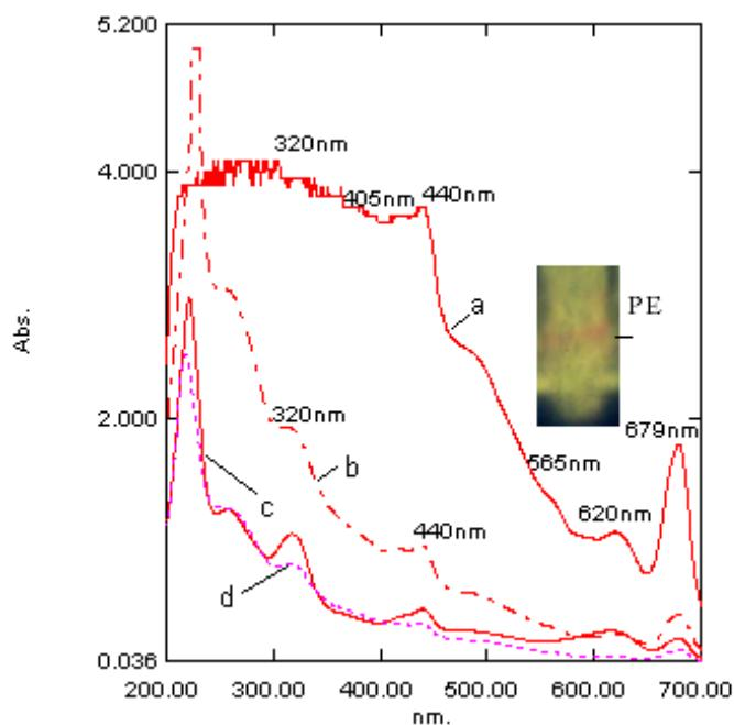
**Supplementary Fig. 2.** UV-visible overlay absorption spectra of cell free enzyme extract (0.5 mg protein ml<sup>-1</sup>) of *L. arboricola* having at each step of purification. (a) crude extract, (b) 60% acetone precipitation (c) after ethanol: chloroform treatment, (d) after ion exchange chromatography . (Inset: native-PAGE of catalase isoforms along with PE in the cell-free extract of the cyanobacterium).
